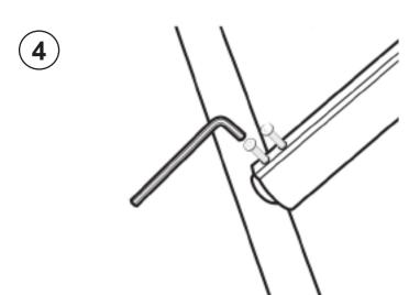
Secure base with allen wrench and two screws
